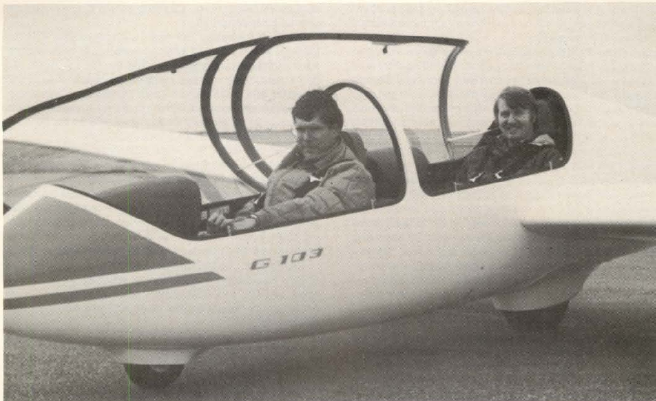
Cockpits have separate canopies with improved latches. Mike Newgard (rear cockpit) assisted with airspeed calibration tests. 6' 3" test assistant Bruce Beddow fits easily in the front cockpit.
