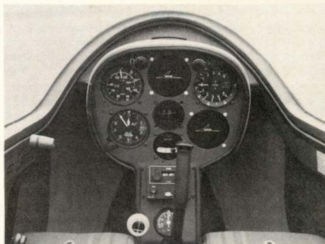
Uncluttered front cockpit with air/wheel brake lever on left side; tow release at lower left side of instrument panel pedestal.
